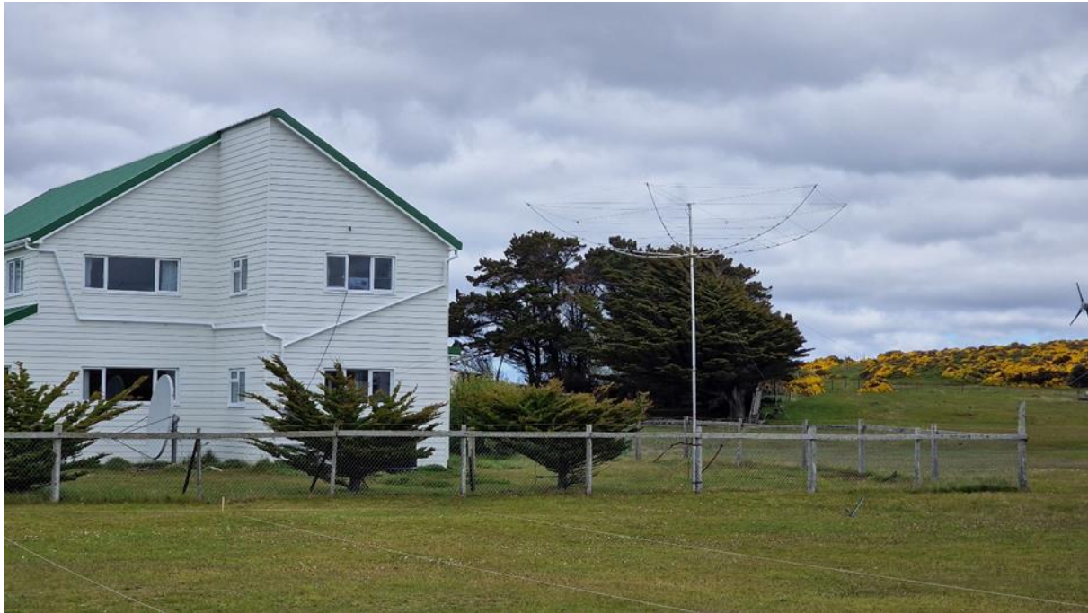
Figure 9 - Hexbeam on an approx. 5m tall mast which was fixed with straps to a pole of the fence.
