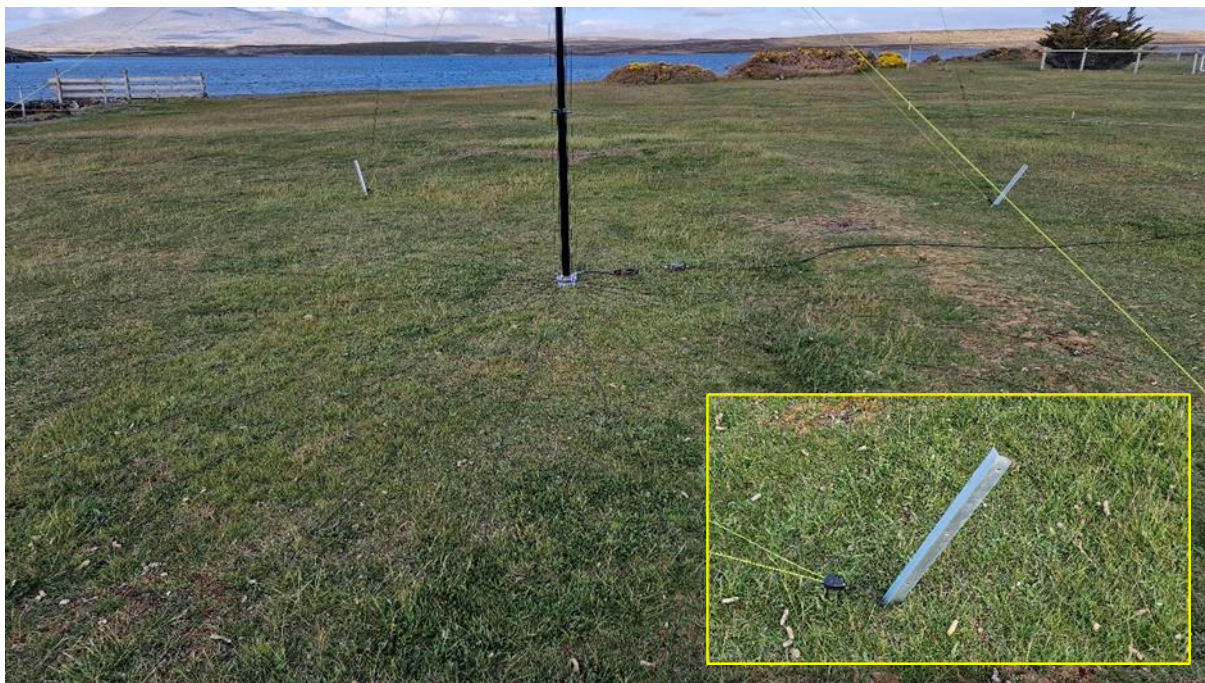
Figure 6 - 32 radials, 3.5 meters long and extra-large guy anchors.
