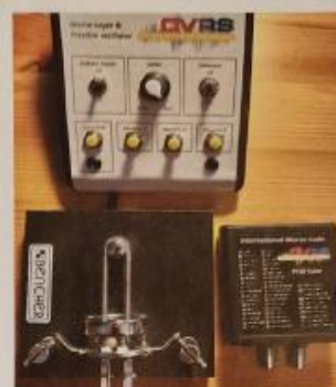
PHOTO 2: CVRS Morse keyer, oscillator and tutor.
