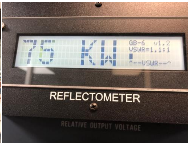
The antennas are well constructed & fed with minimal-loss open feed line. Note SWR of 1.1:1 at 75,000 watts ! (QRP Power for GB-6)
