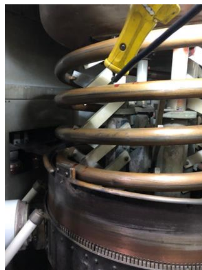
Right: Tuning coils for finals - note the entire tube config is on a rotator.
