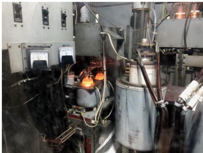
Old fashioned tubes that will fry you; Note Plate voltage of 13 KV.
