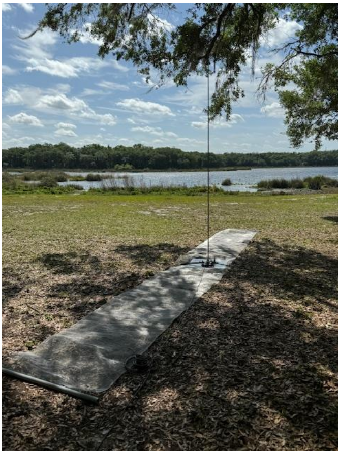
Wolf River Coil with 17 ft whip on top of a "magic carpet" ground plane. Yes, it works!
