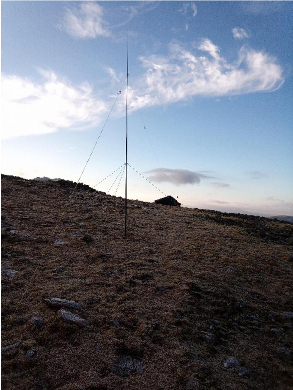
End fed Half Wave for 40 m ,as a sloping antenna using a 6m pole. The 49:1 balun is located at the tent
