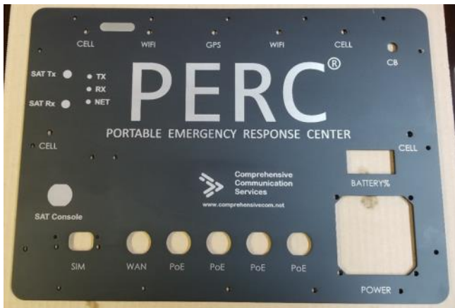
Figure 12 - Faceplate for PERC/SAT GoKit
