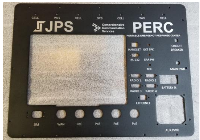
Figure 13 - Faceplate for PERC / JPS ACU-M 1000 - Interoperability Gateway/VoIP/RoIP - 4 radio bridge
