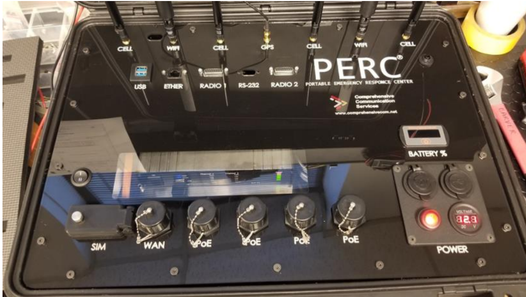
Figure 15 - PERC / JPS RSP-Z2 Interoperability Gateway; 2 radio bridge kit with acrylic faceplate with see through window
