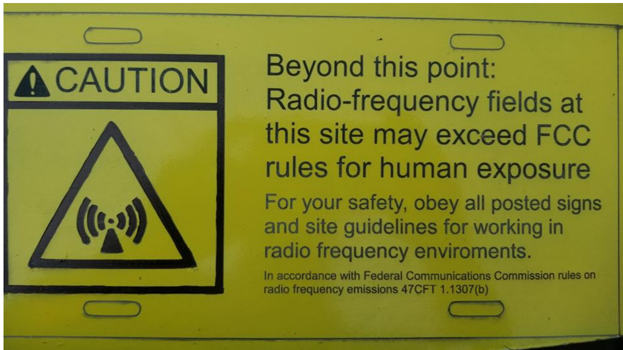
Figure 9 - Aluminum FCC required RF Exposure Warning Sign
