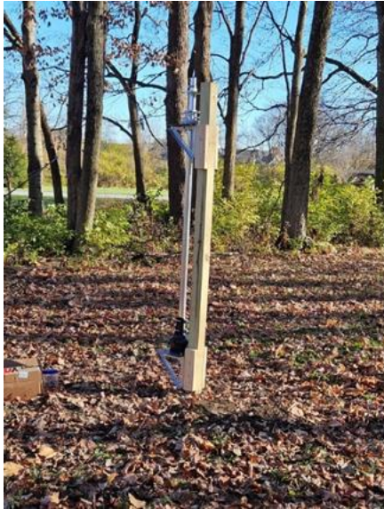
Figure 5 4x4, rotor, and thrust bearing on "tower" portion. Looks crooked but it isn't!
