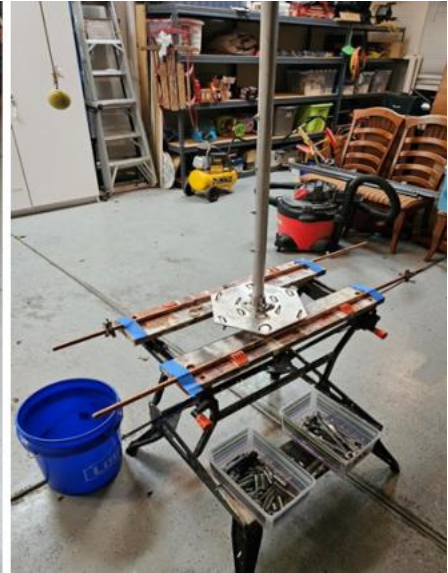
Figure 7 Mast plate and feed point in place - ready for the
