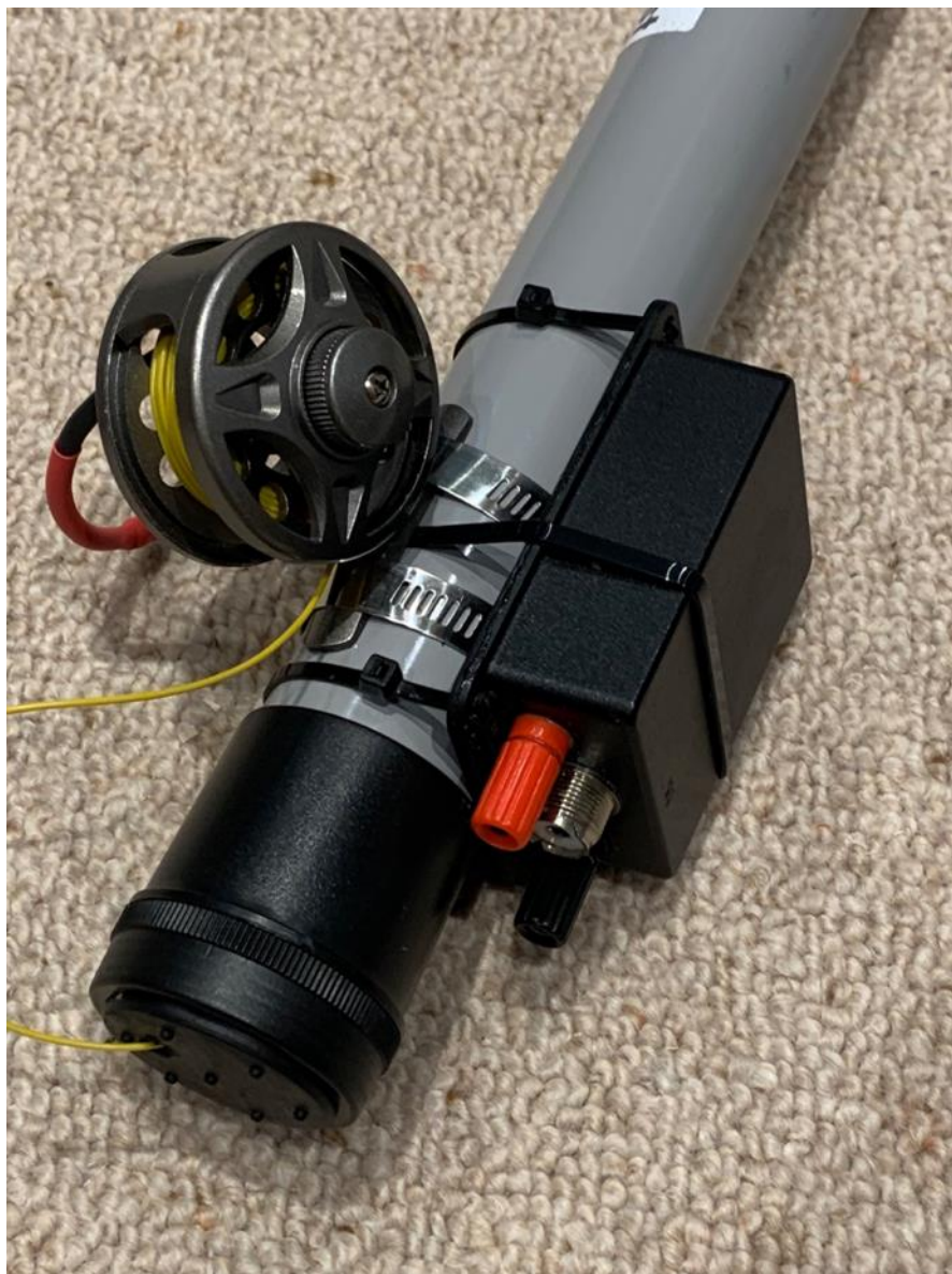
Antenna base with reel of radiator wire and 4:1 UNUN
