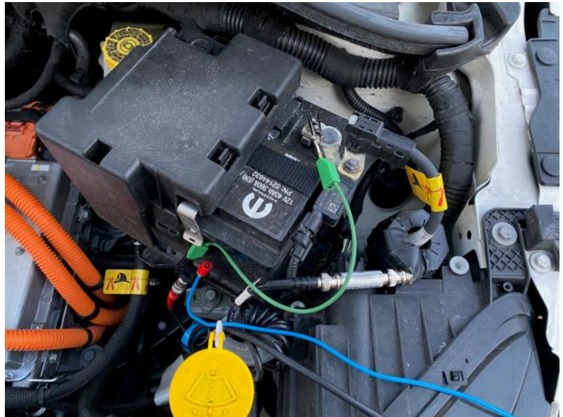
Homemade HF-Current Probe -Snap on ferrite with attenuator on 12V Minus Support Battery Fiat500E
