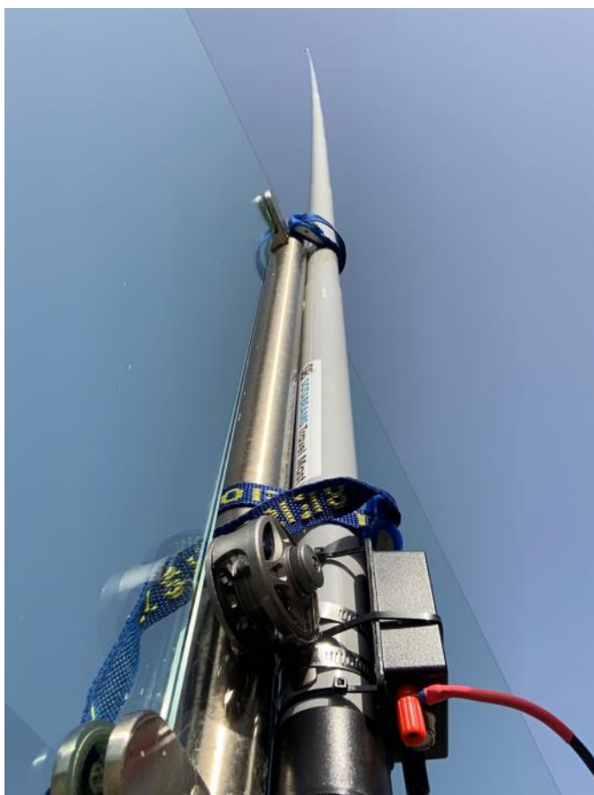
Antenna deployed awaiting connection of coax and counterpoise
