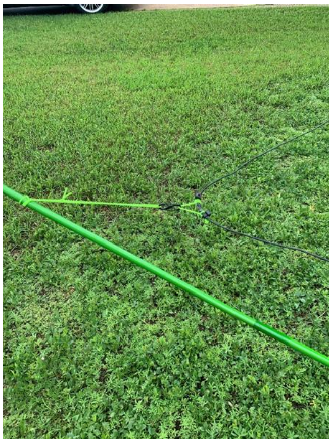
Figure 10 - 15m spreader connection
