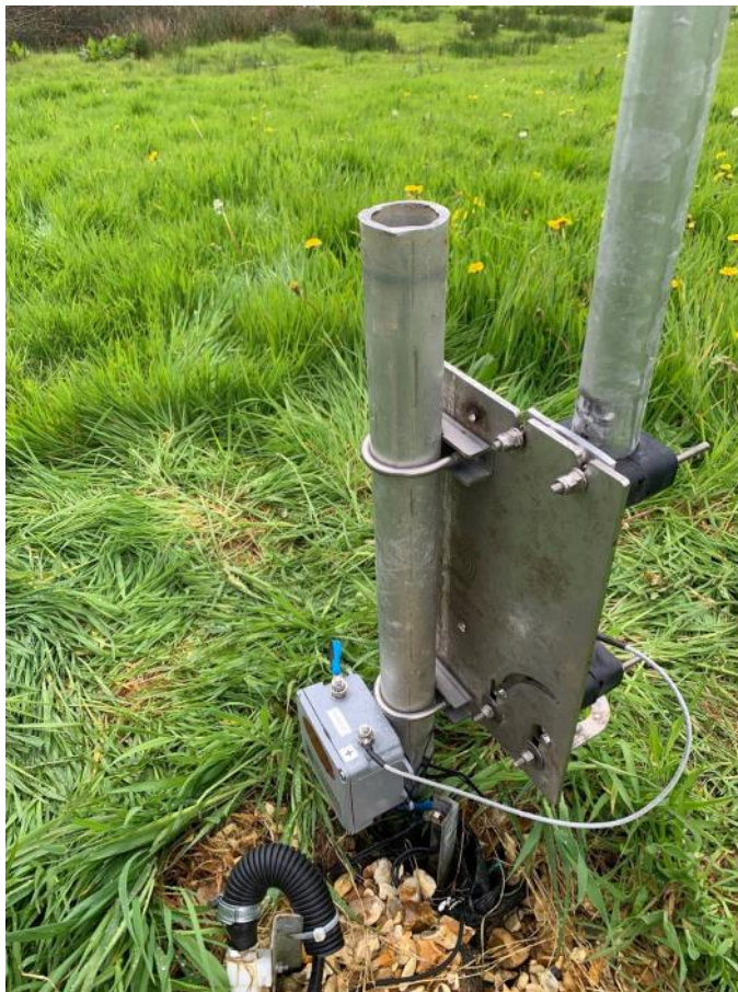
DX Engineering tilt plate and Balun Designs 2:1
