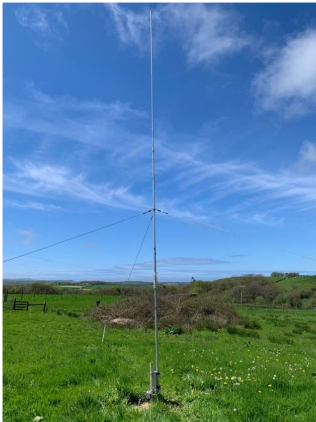
New 40M Vertical using one OB1-40 radiator
