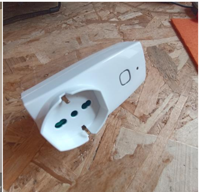
WiFi controlled socket to turn off-on the radio and raspberry power supply
