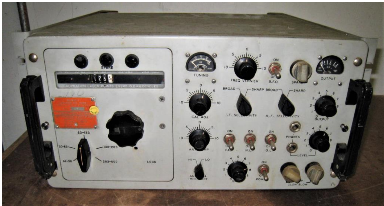
(Above) Navy AN/WRR-3 VLF/LF/MF radio receiver, the same type Chief Decker and I used.
