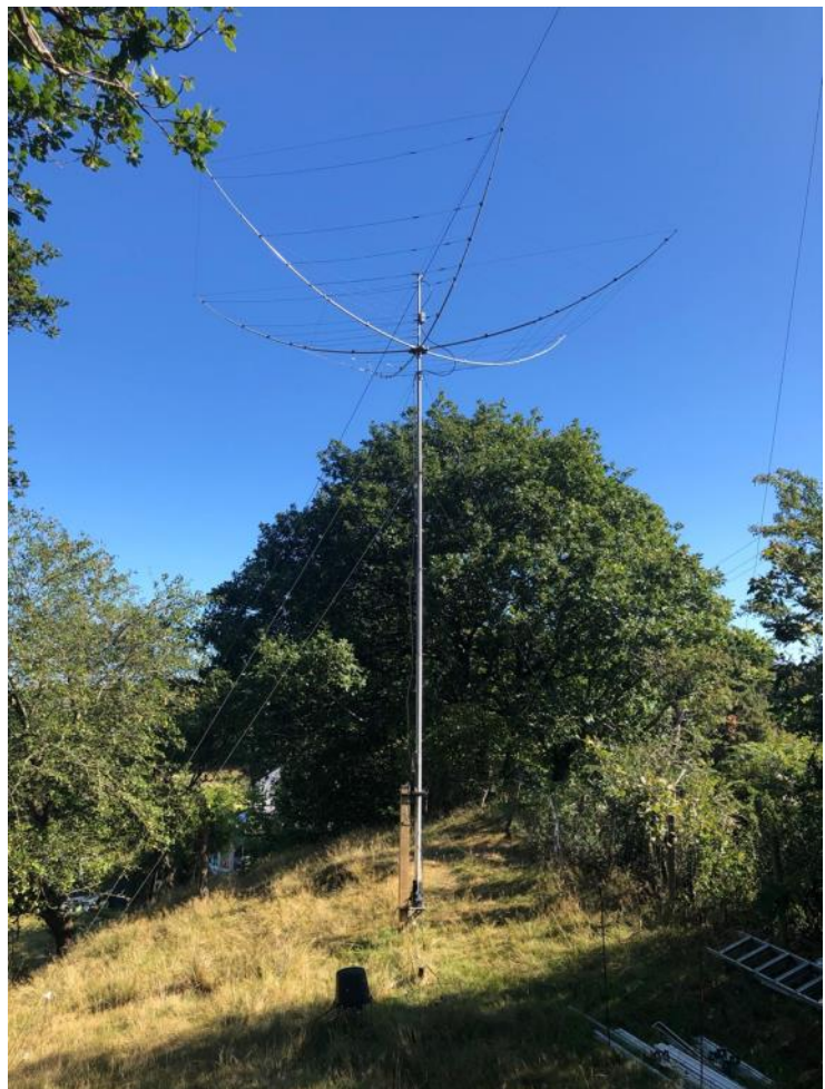
The Hexbeam on mast; note the upturned bucket covering the remote antenna switch!
