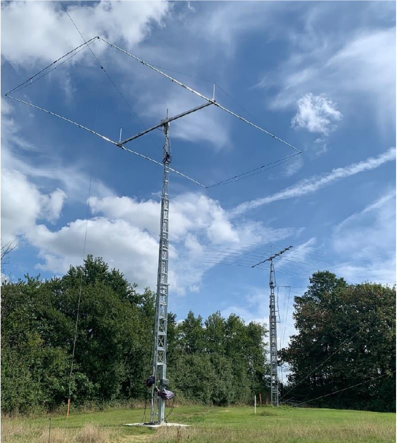
40m Optibeam Moxon on new mast with Optibeam OB9-5 in the background on an identical mast
