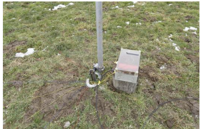
Vertical with tuning unit and about 24 radials.
