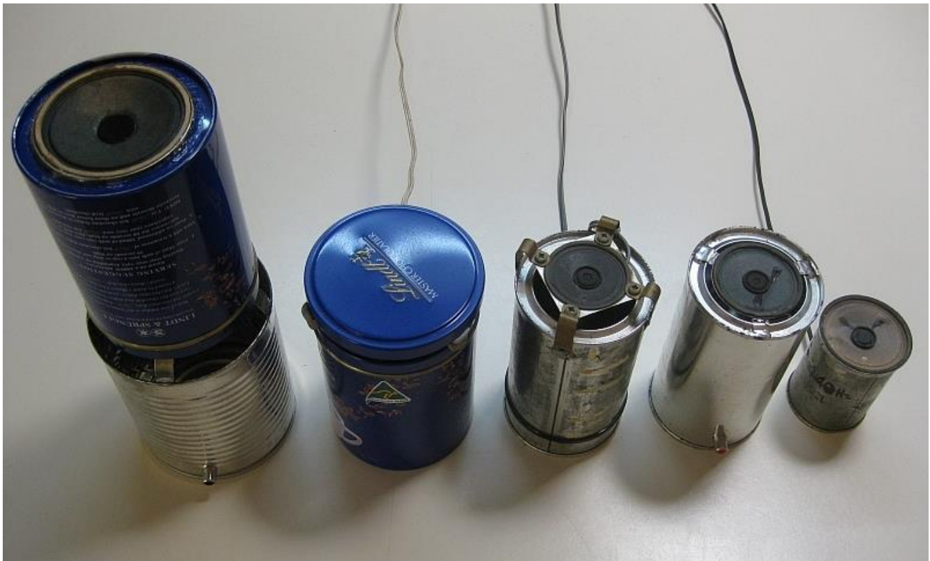
Five VK6GX CanSpeakers, all resonant at 500Hz.
