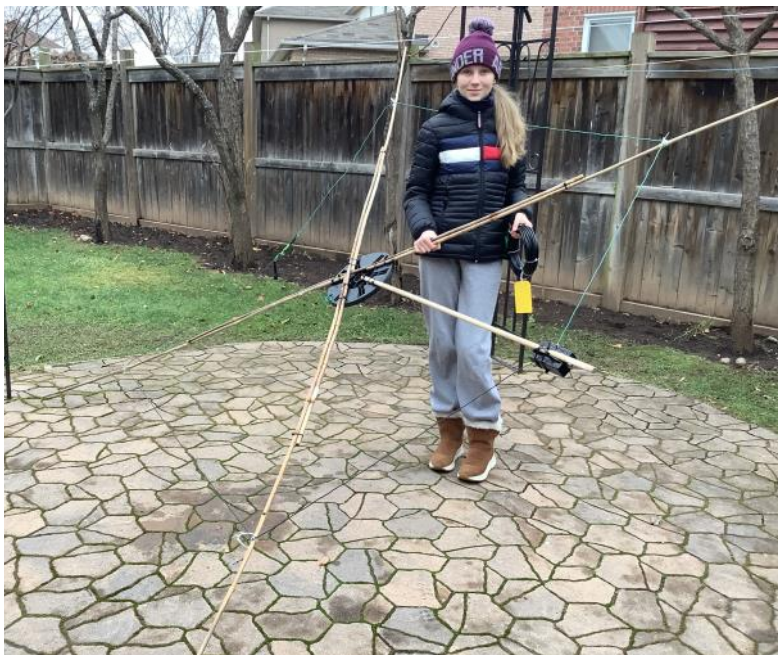
Building a Cobweb antenna prototype for our small city lot.
