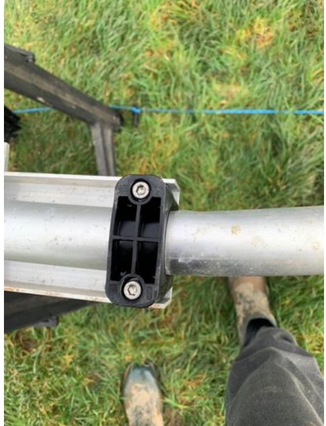
The only damage to the Optibeam: - a slightly bent Driven Element!
