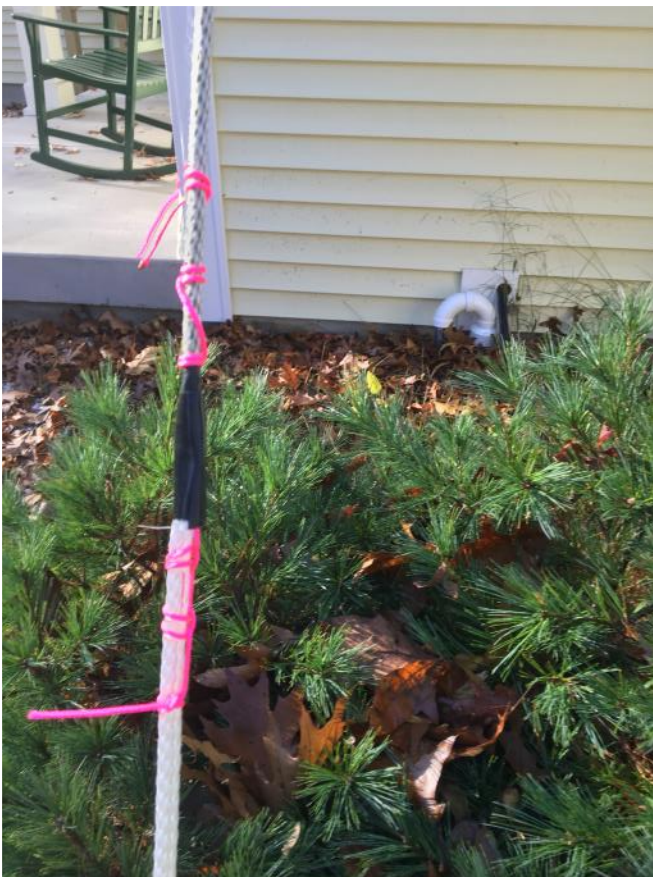
The splice with clove hitches before taping (left) and after taping (right).
