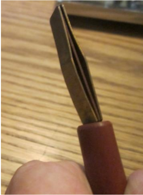
Telephone switchboard plug
