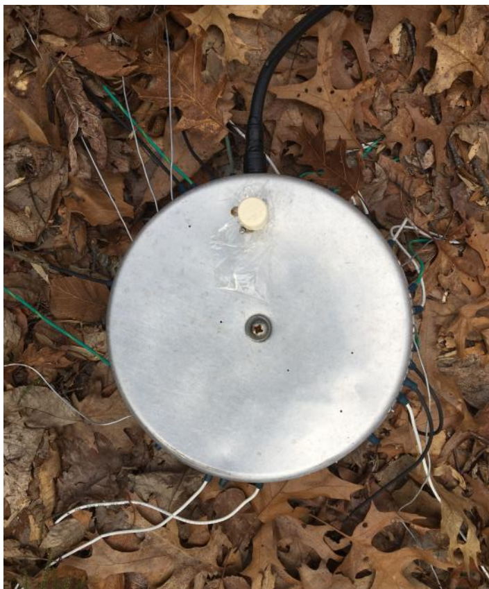
The cake pan radial plate with the vertical wire disconnected. The SO239 connector has been covered with a PVC end cap.
