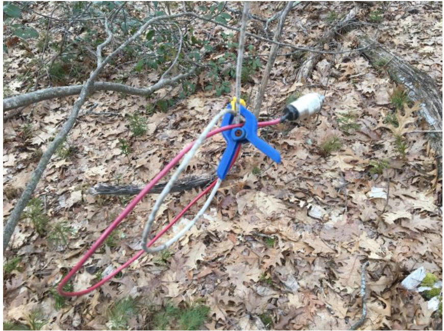
The disconnect vertical wire coil held in place with a spring clamp, ready for wind gusts.
