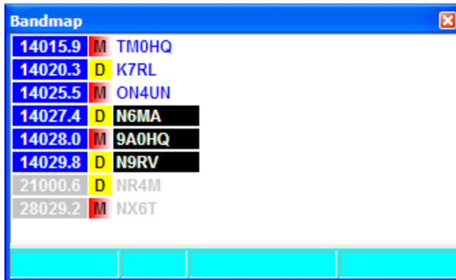
To have the band map filled from a DX cluster select “DX Cluster” under TR4W’s Windows pull down menu. This brings up the DX Cluster window. The upper left box is used to select the cluster you want to connect to. The rest should be familiar if you have ever used a cluster.
