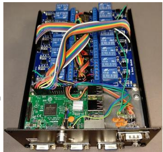
Top: FreqEZ HAT in an Argon Neo case Bottom: DIY FreqEZ construction with Sainsmart relays
