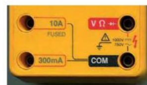
Figure 1 — Voltage ratings are shown next to a voltmeter's probe jacks (1,000 V dc and 750 V ac). Exceeding these voltages can result in a flashover, presenting a severe electrocution hazard.
