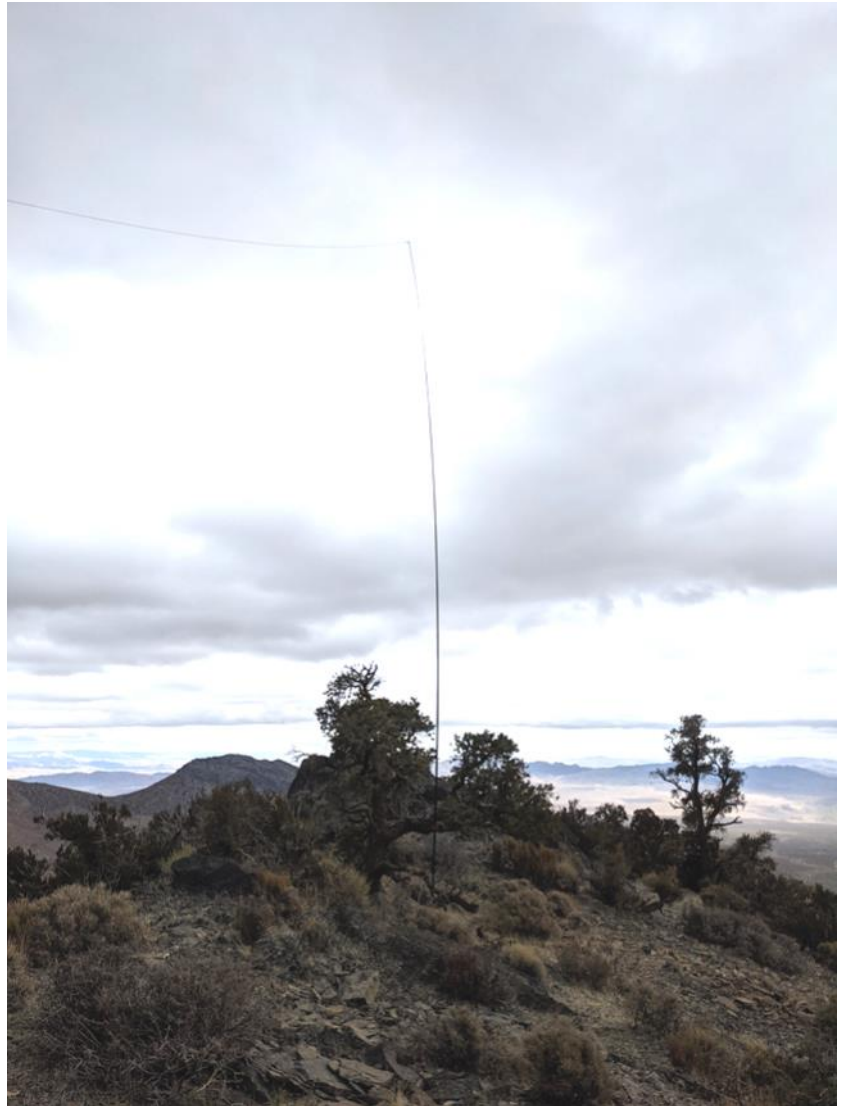
On mount Stirling with telescoping mast and 20 m EFHW
