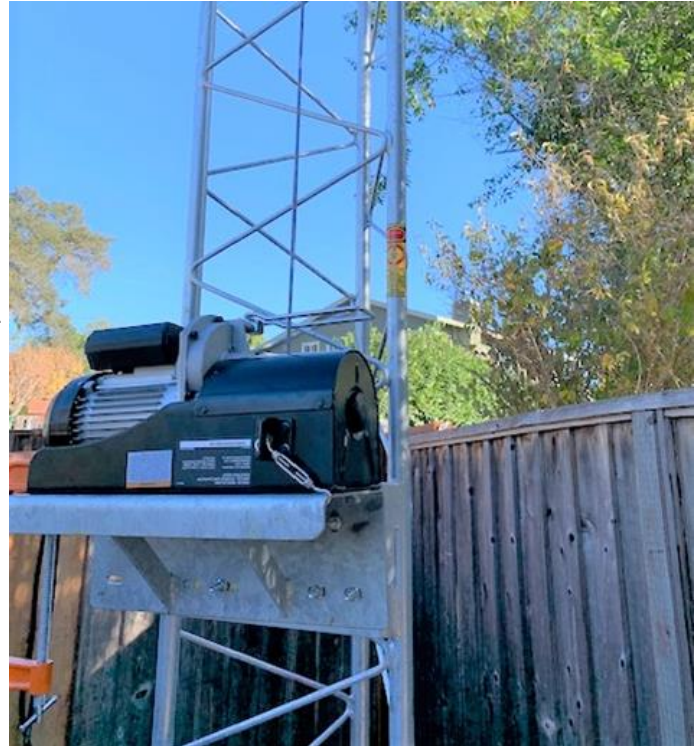
Tower modified by removing hand winch and replacing it with hoist mount and electric hoist system
