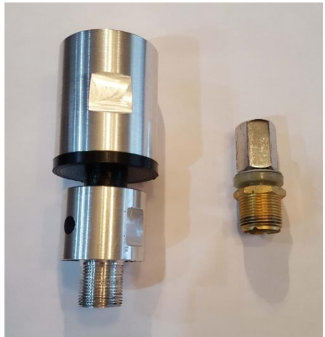
Figure 1 - Comparison of the load bearing area of the two insulators.
