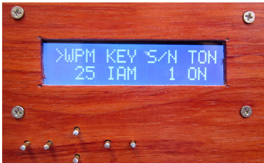
Figure 7: Closeup of the 16x2 LCD Display/Keypad in use. This display indicates operation at 25 WPM, iambic keying mode, QSO serial number set to 001, and sidetone on. The cursor (>) indicates that up/down buttons will adjust WPM. The right/left buttons scroll the whole display to reveal other parameters like sidetone frequency, etc.
