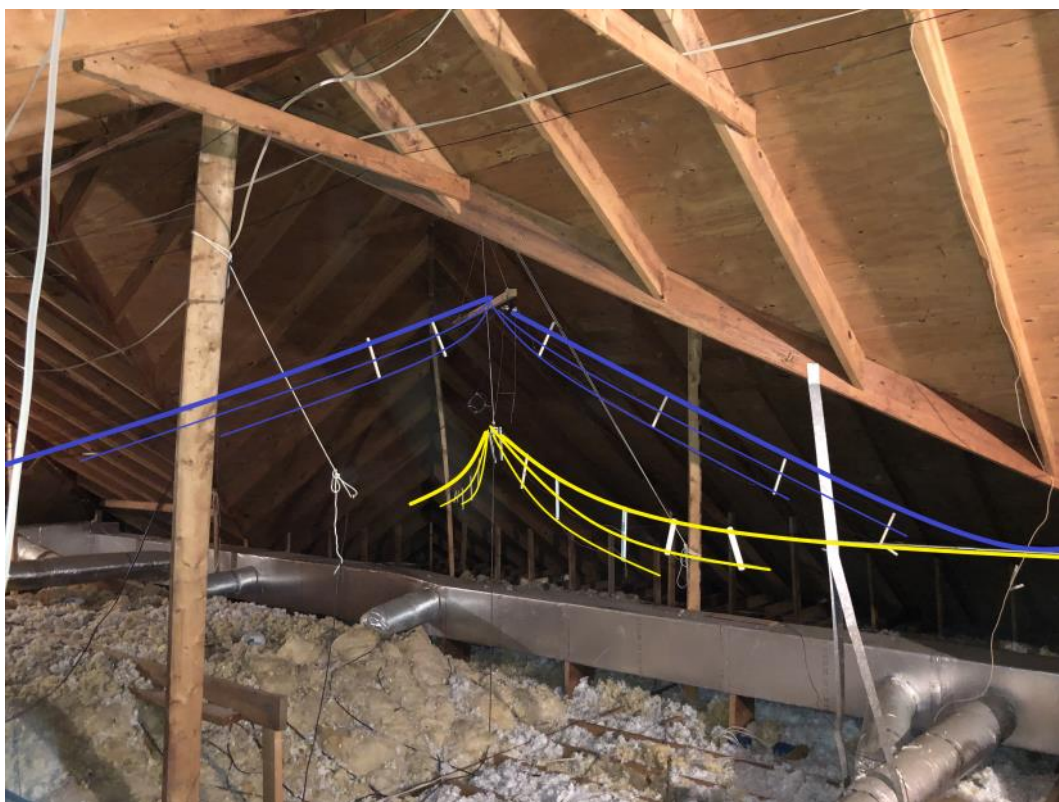
Two triband antennas; the wire Yagi and the fan dipole underneath it along the boom. The dipole is in yellow and the yagi is in blue.
