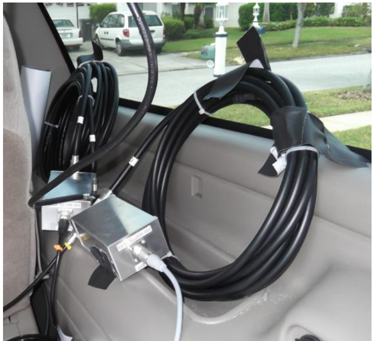
Above: antenna farm. Below: 15 and 20m band pass filters and stubs
