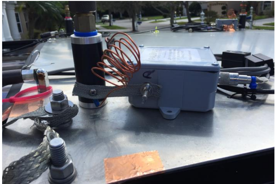
Feedpoint RFI mitigation. Look closely, there's a lot going on.
