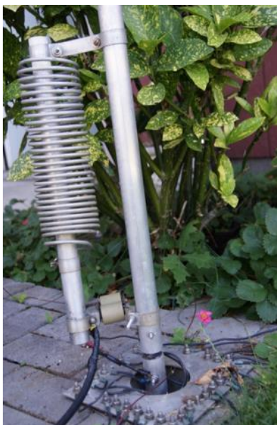
The eBay 160M coil (left) and new cap for the 30M coil.
