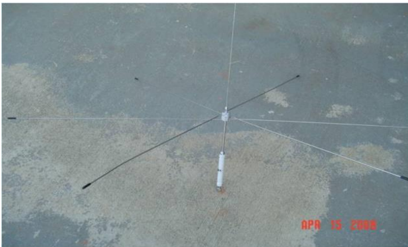
15 meter Hustler Resonator with DX Engineering Hot Rodz Capacity Hat for use on 20 meters
