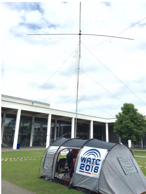
WRTC2018 station was presented. Antennas are a SPiderbeam 10-40m and a 80m dipole
