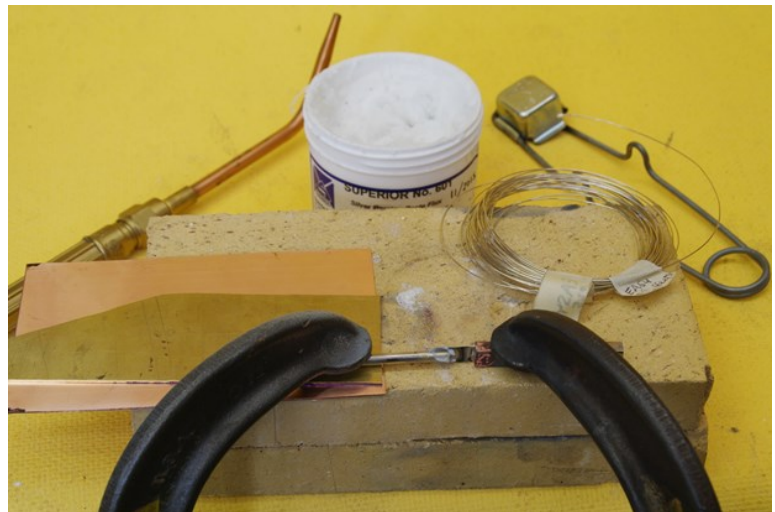
Figure 3. Silver soldering the main spring in a simple fixture.
