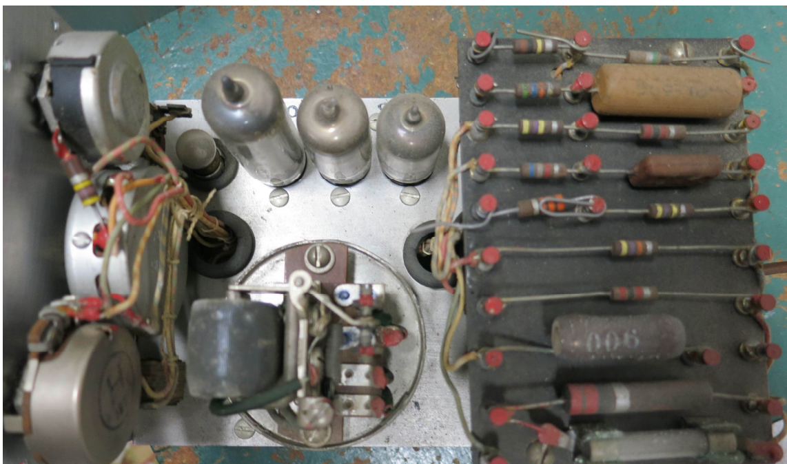
Figure 5. Inside top chassis view, showing the front panel controls, terminal board, tube layout, and relay.
