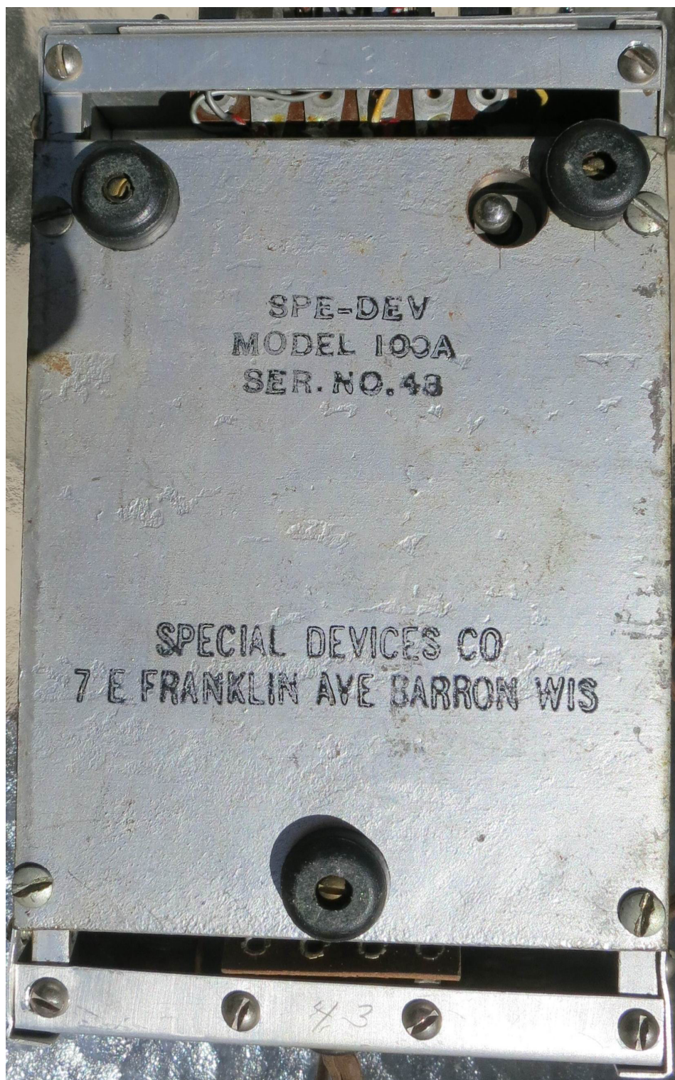
Figure 3. Model 100A bottom plate is made of lead and stamped with the manufacturer and product ID information.
