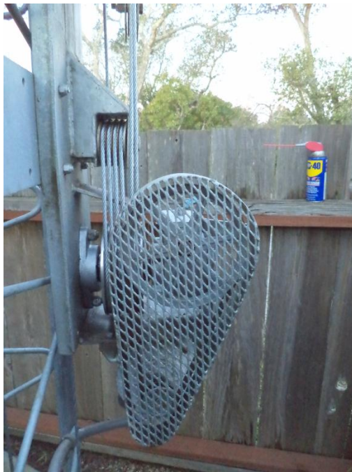
For manual operation, the fan shroud comes off and the crank locks onto the large pulley
