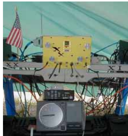
Bridge connects the two tables and supports cabling and the controller box (auto antenna selection with override, BPF drive, keyers, octopus). Power monitor, auto tuner, and rotator are beneath.
