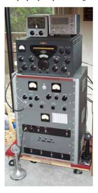
Taming down the Globe King 500 was a real challenge. It is cathode keyed and had virtually no key shaping. To say it was a "click monster" is gross understatement. But, even the grid-block keyed Ranger and Valiant could be key shaped by playing with the values of R and C in the keying circuit. Have any of you done some of that? If so, let me know, it could be the kernel of an interesting future piece.
